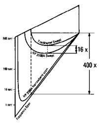
Traditional swept analyzers trade off measurement speed for accuracy.
