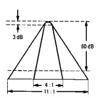
Three technological breakthroughs result in faster measurements: improved shape factor, oversweep compensation and narrowband zoom mode.
